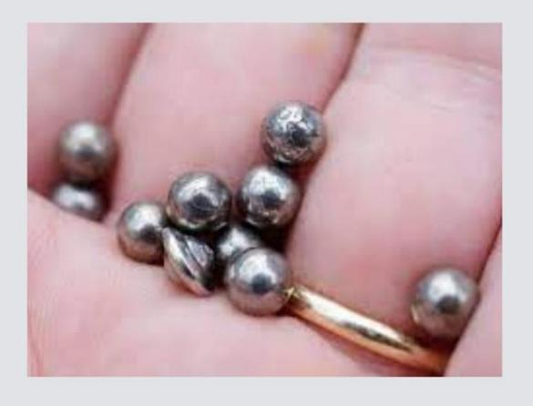
It's important to note that steel shots and grits are significantly more cost-effective than aluminum or ceramic abrasives because they have much longer life spans and less easily wear down due to their high density properties.
