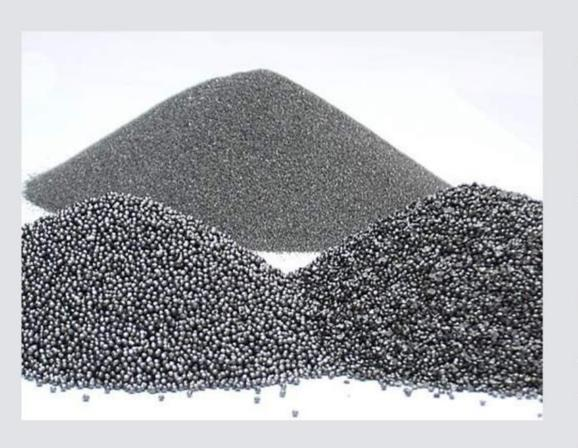
These particles are then ground into smaller sizes and mixed with water to create slurry. This slurry is poured into molds made from sandstone. which are used for sintering by heating them up to 1,400 degrees Fahrenheit (760 degrees Celsius). After cooling down for a few hours, these molds are broken open to reveal steel shots and grits.
