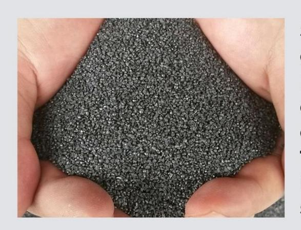
Steel shots are used primarily in grinding and polishing applications, but can also be found in cutting or drilling applications where a high degree of surface finish is required. The industrial uses for steel shots include grinding and honing steel, stone and other materials.
